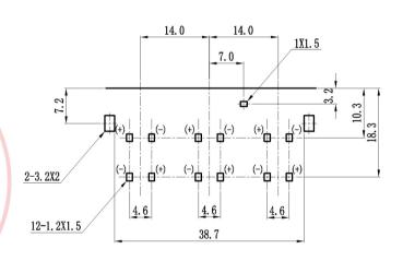
PCB MOUNTING HOLES (Solder surface)
