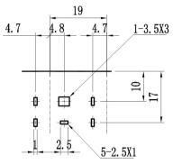
PCB MTG (Solder surface)
