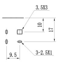
PCB MTG (Solder surface)
