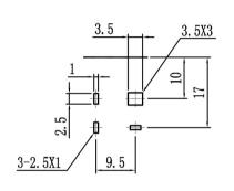
$\frac{\text{PCB MTG}}{\text{(Solder surface)}}$  TOP VIEW
